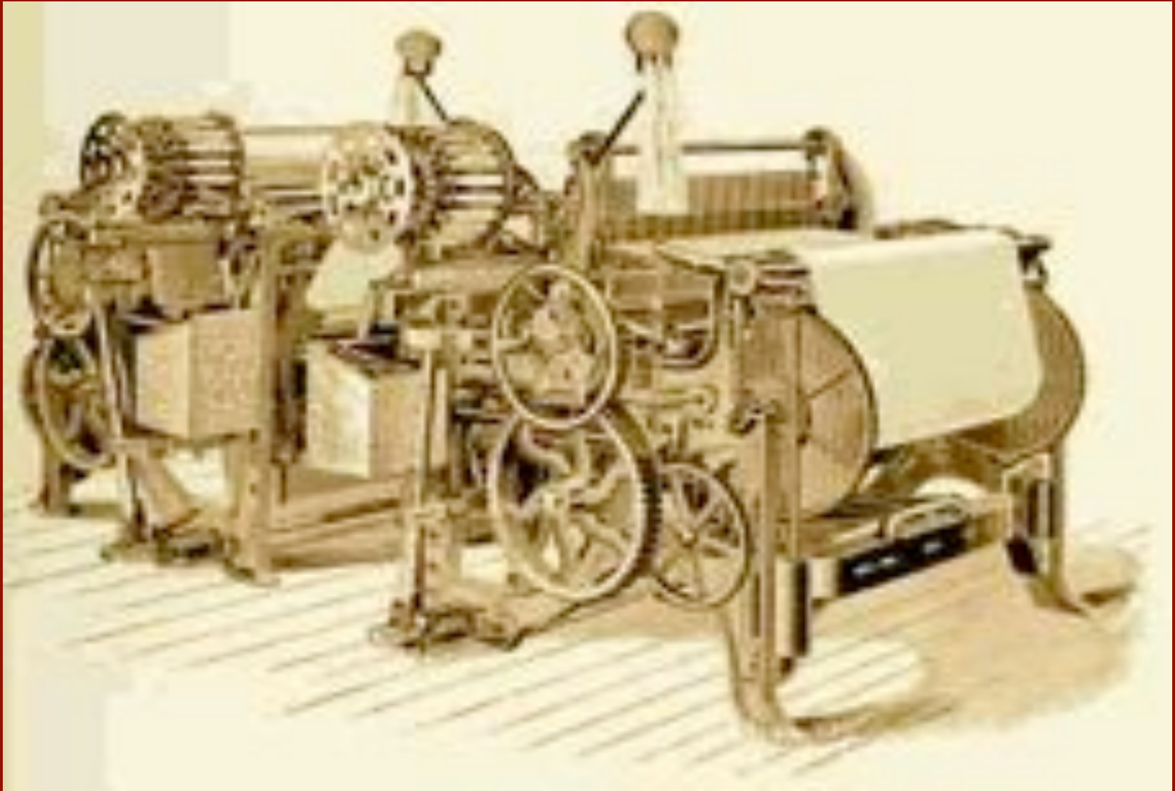
Model "A" Northrop Loom, 1894
